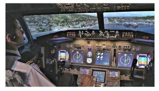
In this example, the instruments in front of the pilot are real and the windows are screens displaying virtual content.
