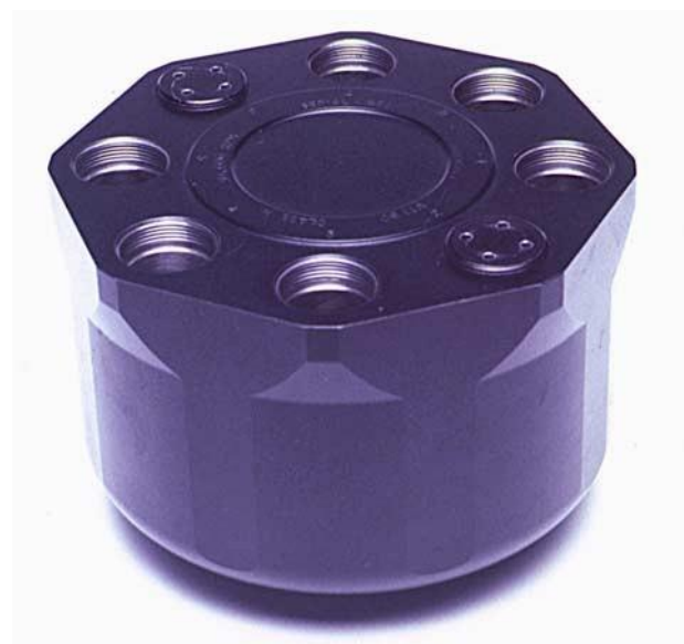
Figure 7 A vertical tube rotor.
