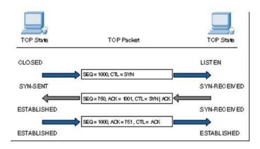
After the connection has been established, the TCP protocol manages the reliable exchange of data between the two systems. The algorithms that determine the various retransmission timers have been redefined numerous times.
