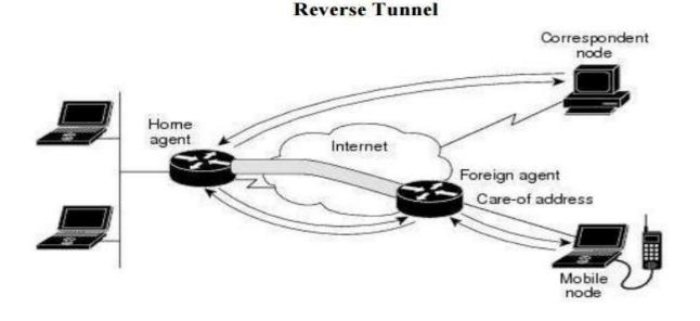
Tunnel MTU discovery is a mechanism for a tunnel encapsulator such as the Home Agent to participate in path MTU discovery to avoid any packet fragmentation in the routing path between a Correspondent Node and Mobile Node.
