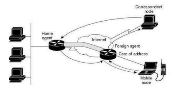
However, this data path is topologically incorrect because it does not reflect the true IP network source for the data — rather, it reflects the home network of the Mobile Node.
