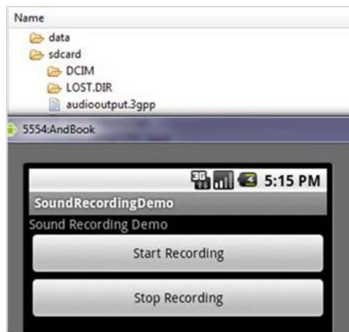
Figure 10.6. An example of audio files being saved to the SD card image in the emulator
