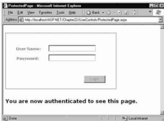
Figure 22-6: Using the LoginBox user control
